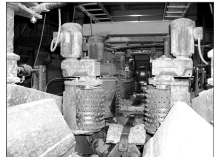
Figure 2. Tilt roll log rotator with two pairs of tilts (Heinola Sawmill Machinery)
