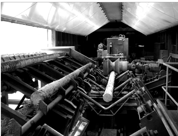
Figure 6. Automatic log rotator with real time measuring and optimization (Genera)
